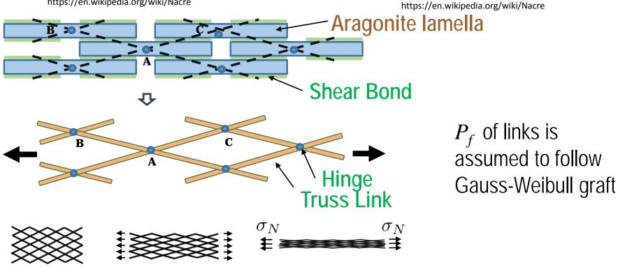
Collapsed (for computations) No Load Mechanism
