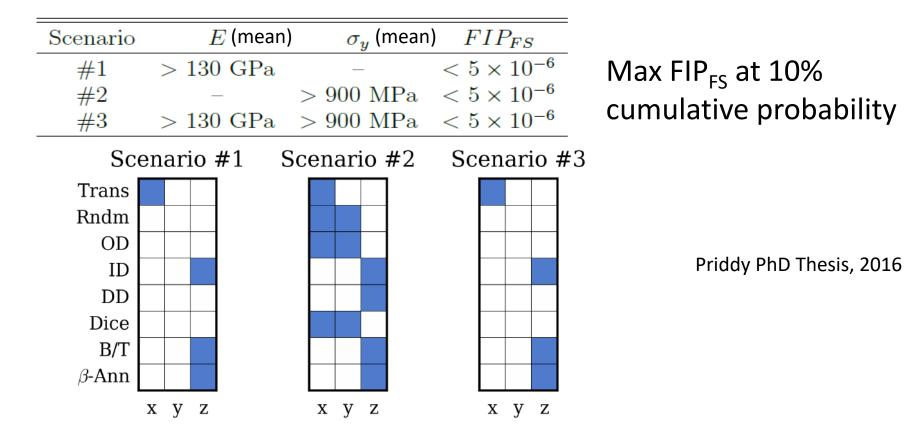
Two-dimensional representation of the feasible space for each of the design space for each design scenario applied to each of the 8 textures and 3 loading directions. Blue boxes indicate satisfaction of the performance requirements.
